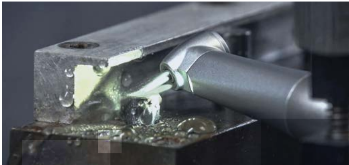
Test of retention force of the bur with more than 3 kilograms
