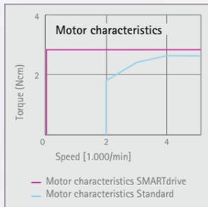
Leverage the high torque and vibration-free start-up characteristics of your KaVo SMARTdrive with its extended speed range of 100 - 40,000 rpm.
